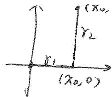
$$\int_{r_1} \vec{F} \cdot d\vec{s} = \int_0^{x_0} \begin{pmatrix} 4 \\ 3t^2 + 4t \end{pmatrix} \cdot \begin{pmatrix} 1 \\ 0 \end{pmatrix} \cdot dt = 4x_0$$
